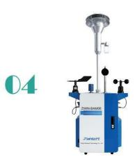
BAM1006 Continuous Particulate Monitor adopts the principle of  $\beta$  ray attenuation to measure the particle concentration. The result is accurate and reliable. It consists of three basic components: the instrument host, the cutting head, and sampling system.
